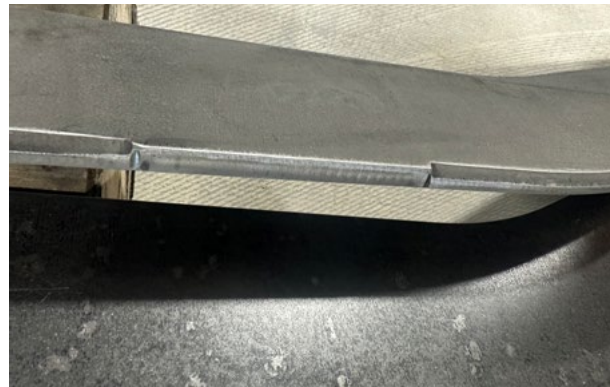
Compound bevel cut combining Top Y bevel and straight cut on the same geometry
